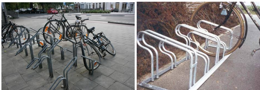
Horizontal front-wheel grips are TO BE AVOIDED (image source: T. Asperges)
