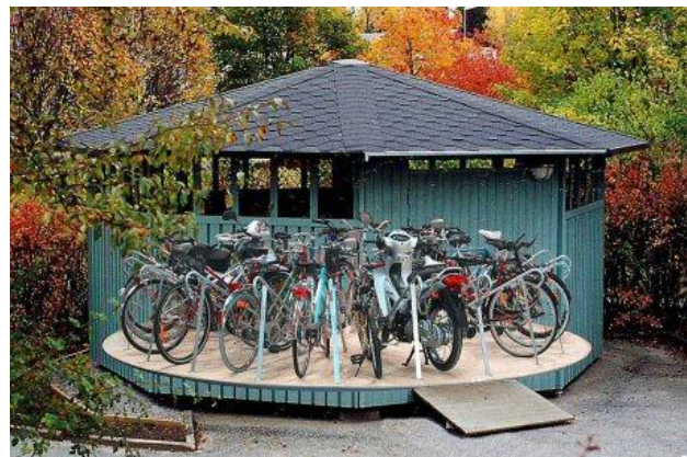
Carousel cycle locker: bicycles are on hand-rotated platform that moves your bicycle in front of the single-door entrance (Sweden, see clip on www.plugin.se )
