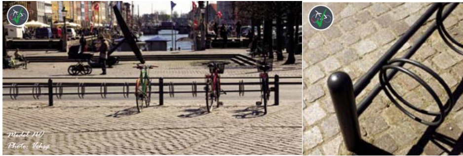
Vertical front-wheel grips, common in Denmark (image source: P. Celis – 2008, Bicycle Parking Manua, DK )
